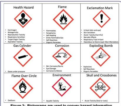
Figure 3: Pictograms are used to convey hazard information in an easy to understand format.
